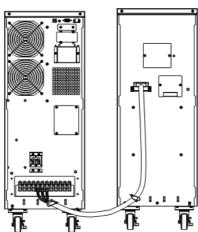
Step 4: Rotate the battery cable retention bracket and tighten the screws to fix battery cable.
