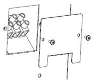
Step 2: Connect the Battery Cable to the battery input Terminal Block and ensure the polarity is right, then retighten the Block Cover.
