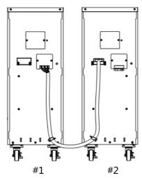
Step 5: Rotate the battery cable retention bracket and tighten the screws to fix battery cable.
