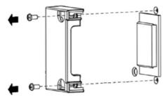
Step 3: Connect the Battery Cable to the Battery module.
