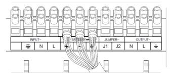
Step 2: Loosen the screws to remove the battery cable retention bracket of the Battery module.
