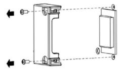
Step 4: Connect the #1 Battery module to the #2 Battery module.
