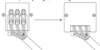
Step 3: Loosen the screws to remove the battery cable retention
